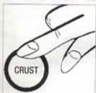
indicates the appropriate colour selection. When the bread mode is selected. crust colour defaults to Medium, Press 'CRUST' button once for Dark and twice for Light.
